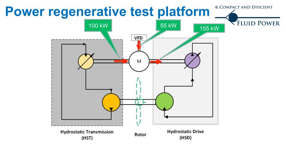
> To Investigate the performance of hydrostatic transmission
