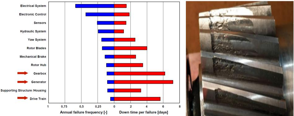
Failure frequency and downtimes of components
