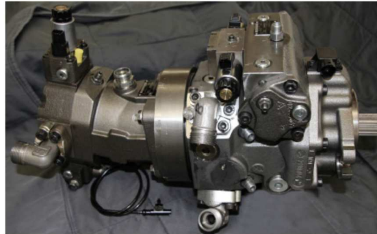
Fig. 2: test unit (tandem unit - A4VG pump / A6VM motor)
