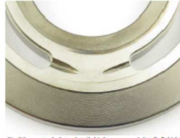
Fig.56: control plate detail high pressure inlet (left kidney)
