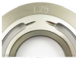
Fig.55: control plate detail high pressure outlet (left kidney)
