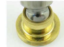
Fig.58: slipper pad retaining plate side
