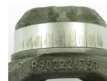
Fig.61: cradle bearing low pressure side
